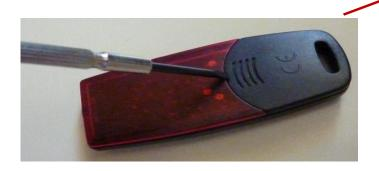
Insert two CR2016 3V batteries with the writing on the battery facing down. Note: there is a silver lug which both batteries must sit in front of so they touch the circuit board
